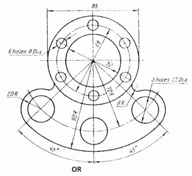
Q.1(B) Draw the below figure using Auto CAD commands and dimension it.
